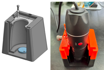
Figure 20: Desk top digital microscope scanner mount and observation table with micro adjustments
