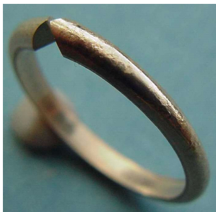
Figure 13: 'Orange peel' surface on a gold alloy ring (Courtesy U Klotz).
