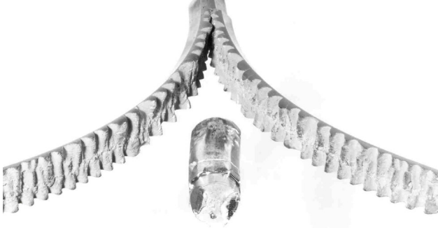
Figure 8: Splitting of gold alloy ingot down the center during rolling ('alligatoring')
