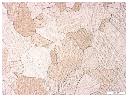
Figure 22: As cast structure of a 950 palladium alloy
