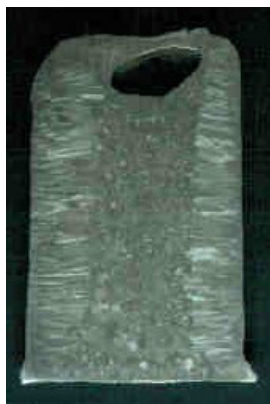
Figure 10: Section of a cast silver ingot showing internal cavity (pipe) and grain structure.
