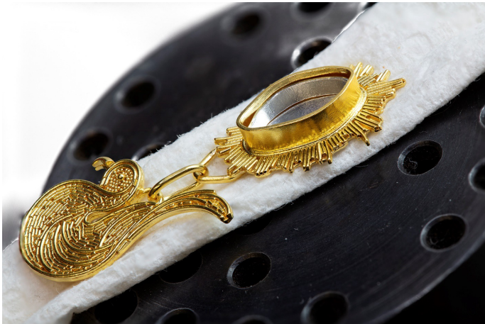
Figure 27: Sheet placed beneath the inner bezel
