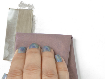
Figure 21: Sanding one side of the sheet
