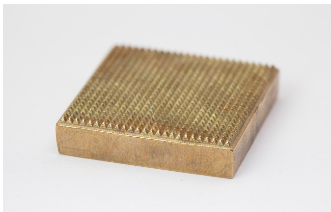
Figure 28: Bronze texture die prototype
