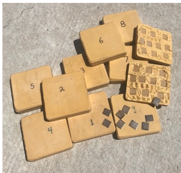
Figure 2: All 10 specimens were vulcanized in each of the 10 molds
