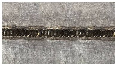
Good weld bead pattern
