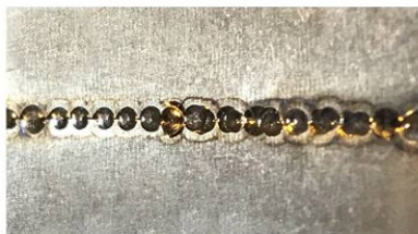
Irregular weld bead pattern
