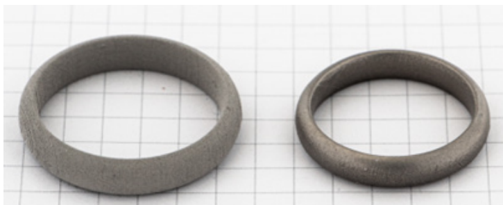
Figure 13: green and as sintered wedding bands in platinum 950 alloy produced by BJT
