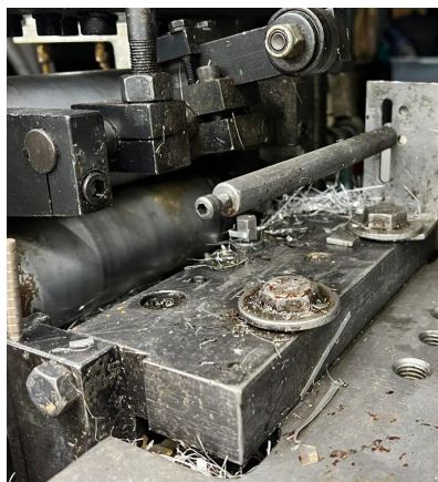
Figure 4: Scrap produced by unacceptable camber (image courtesy of Gold Industrial Machinery Co.)
