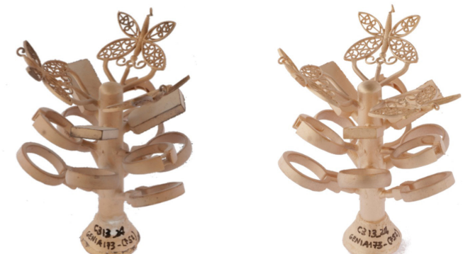
Figure 14: Appearance of refined red gold 18K (r-RG) before and after pickling.
