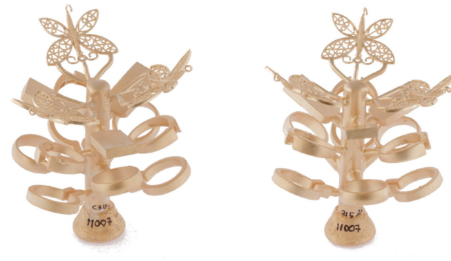
Figure 15: Appearance of red gold 18K with silicon (A) before and after pickling.
