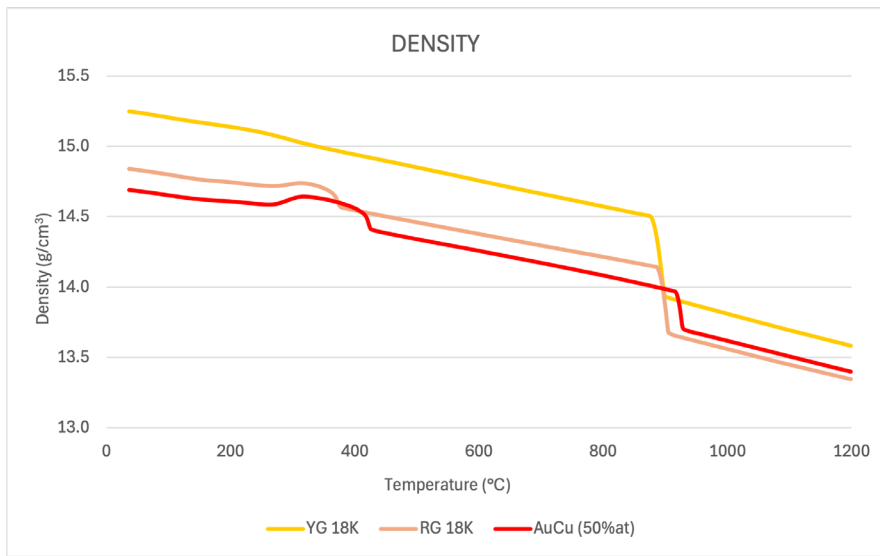
Figure 1: Density as function of temperature in 18K red and yellow golds
