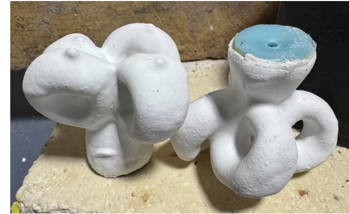
Figure 16: The shells in the green state are fully built with the final seal coat.
