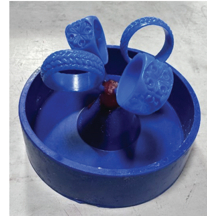
Figure 1: An example of a conventional wax set-up on a rubber base
