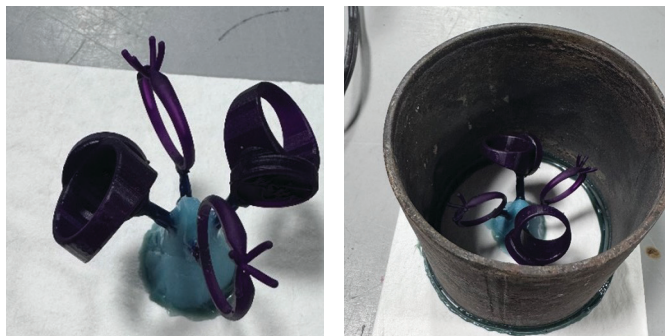
Figure 9: Both images show an example of a conventional setup with resin patterns on a wax button and absorbent paper base. Right: metal flask attached to the absorbent base with wax
