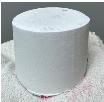
Figure 4: The dental phosphate bonded flaskless mold with the top and bottom trimmed before entering the oven
