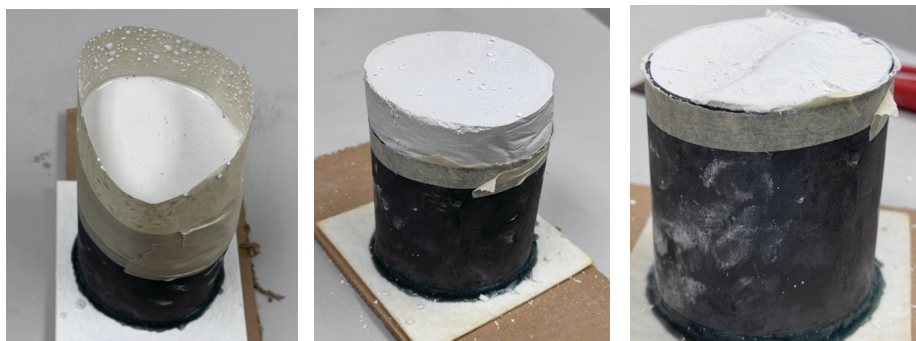
Figure 10: Left: the layer of liquid formed at the top of the set investment; center: after the excess liquid is decanted and the collar removed; right: after the excess investment is removed from the top of the flask.
