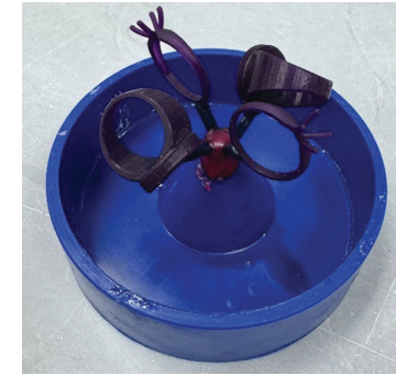
Figure 3: An example of a conventional setup with resin patterns on a rubber base
