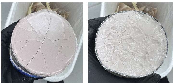
Figure 7: Both images show the ethyl silicate mold after it has set. Left: The gelled and cracked top layer; Right: the mold after the top layer has been peeled away.
