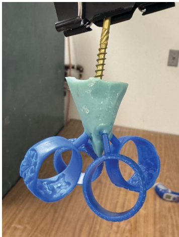
Figure 15: An example of a conventional set-up with wax patterns on a wax base. There is a screw placed into the wax base as something to hold onto during dipping.
