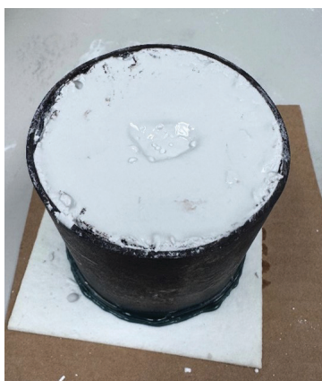
Figure 13: The mold after it has set, with a still glossy surface, as the mold does not appear traditionally set
