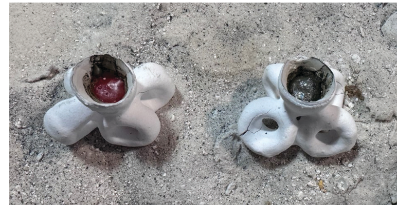
Figure 18: The shell mold after the metal was cast
