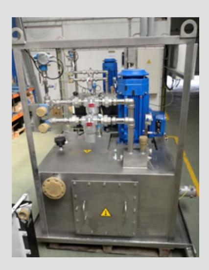
**Transfer Pumps** require high viscosity Lube Oil, lubricating separate points, with specific flow each. **ATC test them running**, during FAT in our facilities
