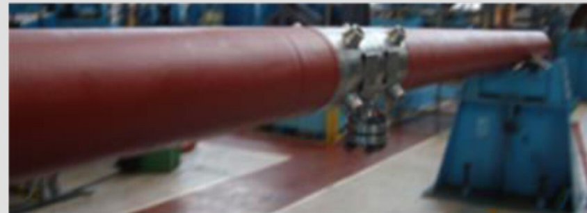
ATC's Calibrated ASME 19.5 PTC 6 Flow Nozzle
