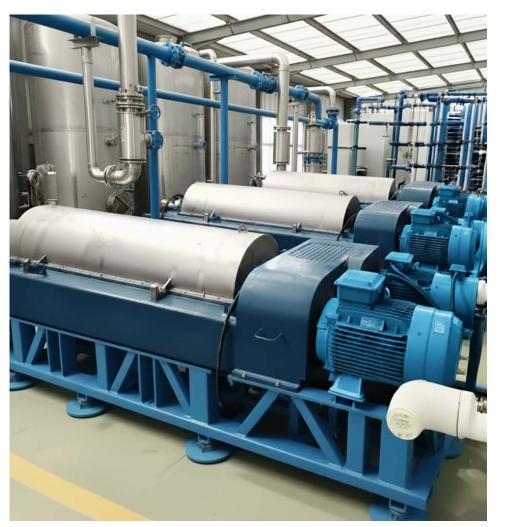
The horizontal screw decanter centrifuge is a widely used piece of equipment for solid-liquid separation at an industrial level. Depending on the characteristics of the material and the specific industry, it can be classified into decanters for dewatering, separation, or clarification. Additionally, with centripetal pump technology, it enables three-phase separation of two liquids and solids, or two liquid phases.
