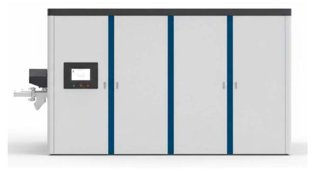
The **thermal evaporation crystallizer** uses steam to evaporate wastewater at 35 °C under negative pressure, producing clear distillate and minimal solid waste. It operates fully automatically, 24/7, as a true zero-liquid-discharge solution. A special scraper prevents scaling by cleaning the tank walls and mixing the wastewater. This improves evaporation efficiency and makes it suitable for new energy, RO reject, concentrate and chemical industries.
