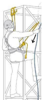
Work restraint (shown below, right) is a technique which makes use of items of PPE to prevent a person from entering an area where a risk of a fall from a height exists. What this means is that the worker is effectively tethered via an anchor point and line in such a way that he is prevented from
