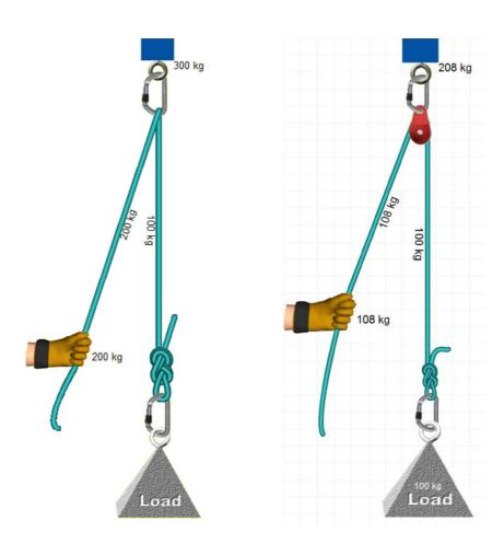
If we anchor the rope above the load and add a pulley to the load, a mechanical advantage of 2:1 can be gained. In the first example we have added in 8% for the friction on the pulley. An upward pull has to be used for this so adding in a pulley to the other anchor bolt would give a change of direction only, keeping the ration 2:1 but making the haul easier. The consequence of the efficiency is that twice the amount of rope will need to be used in the system.
