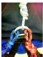
The length of a cow's tail should not be so long that it will be out of reach at full extension. On the cow's tail that carries the back up, the shorter the better. Some manufacturers require a specific length of lanyard to be used with their devices. Always refer to the manufacturers instructions.
