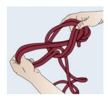
When chain linking a rope you can start from either the middle of the rope or with both ends together, makes no real difference. Begin with a simple slip knot, drop your hand through this loop and pull through another bight of rope. This creates another loop for your hand to drop through. Keep repeating the process until you have reached the end of the rope. Finish by pulling the rope tail through the final loop, this will secure the chain.
