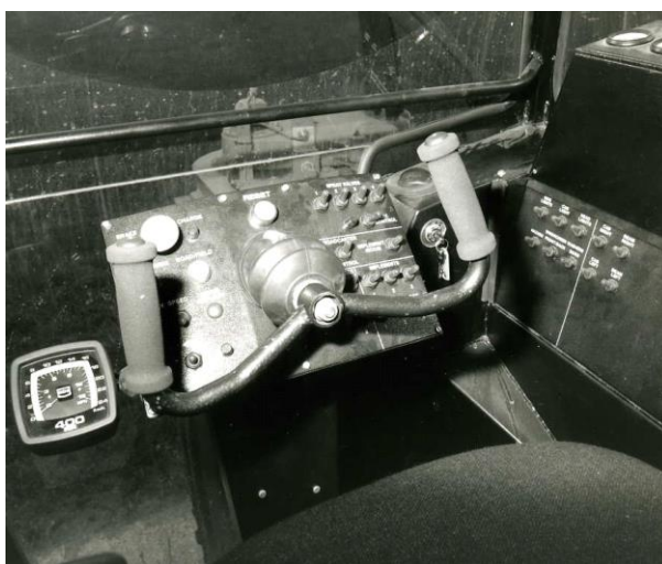
Fig. 16. The steering control column in P5 with ancillary hydraulic controls and services
