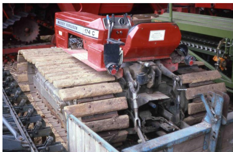
Fig. 2. The Massey Ferguson 174C tracked tractor fitted with wooden cleats. This tractor was used for shallow tillage and drilling across the whole farm
