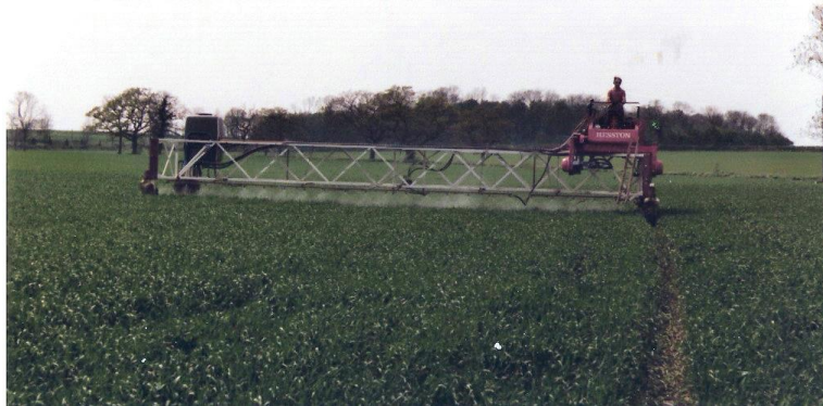
Fig. 1. The first prototype gantry (P1) showing minimum modification of the Hesston swather power unit that was mounted on top of the frame.
