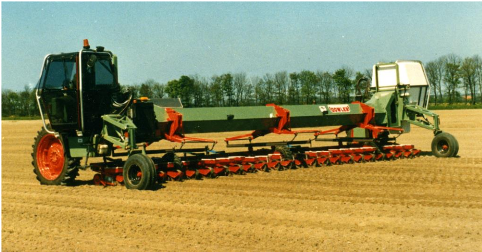
Fig 10. The Dowler P5 purchased by IMAG operating with a 24 unit sugar beet drill
