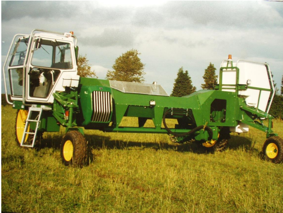
Fig. 12. A 6 m version of P5 that was customised for the University of Hohenheim in Germany. It incorporated a 30 kW power take-off that could be moved laterally on the sub-frame rails.
