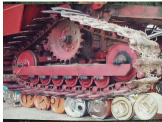
Fig. 3. The harvester on rice tracks demonstrating just how low the ground pressure was beneath them
