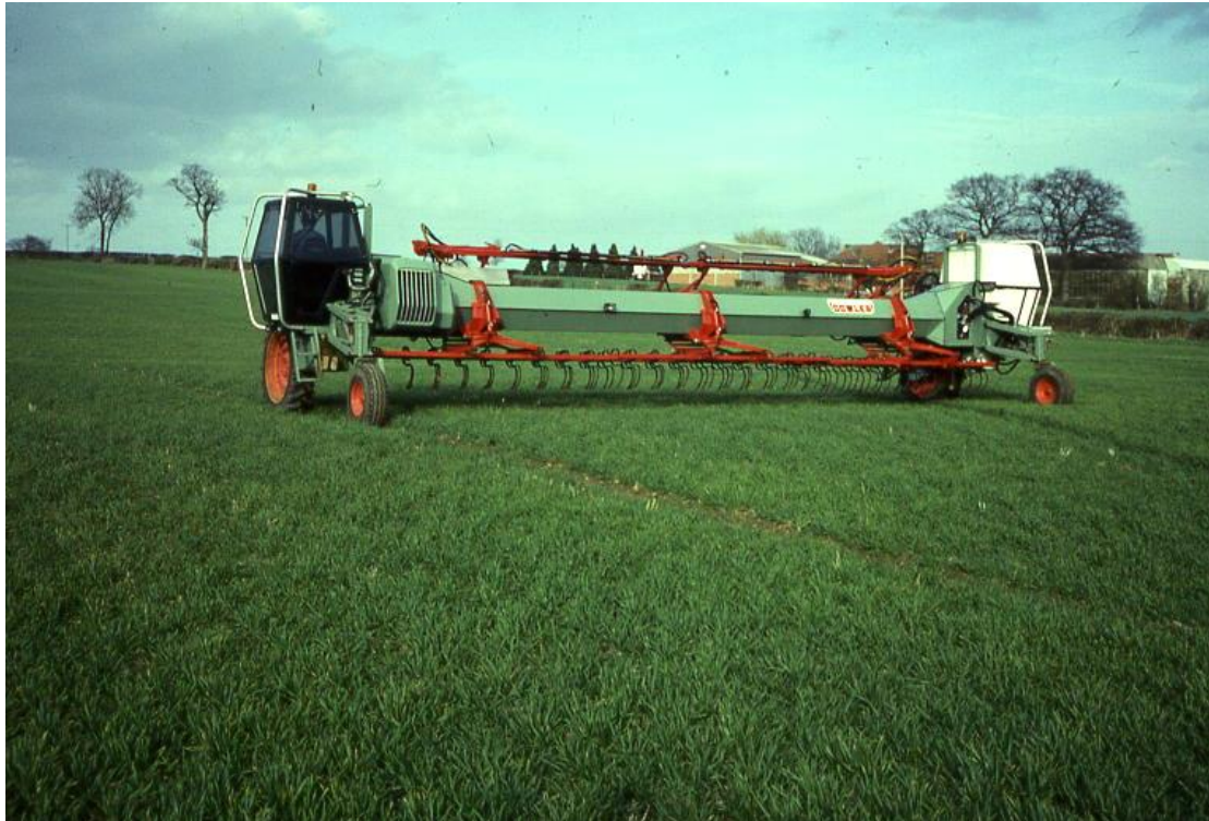
Fig. 11. The production version of the Dowler gantry (P5) showing the attachment of two implements simultaneously, namely spray booms and cultivators
