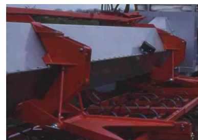
Fig. 8. The two-part hexagon frame showing how the sheets were bolted together and the implement hitch clamped
