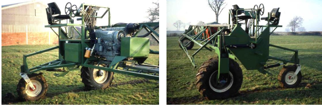
Fig. 5. The driving position of P2 showing the four cylinder Deutz air cooled engine (left) and the mirrored driving positions (right).
