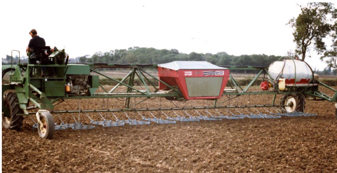
Fig. 4. The second prototype machine (P2). The Nodet fertilizer spreader formed part of the lightweight spanning frame. Upon removal, space frame members were bolted in its place.
