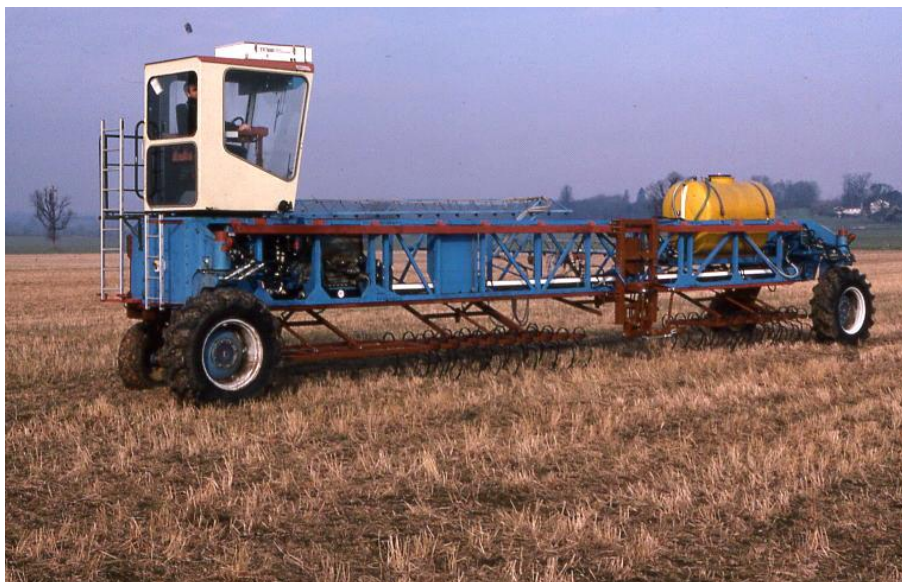
Fig. 6. The Countridge "Monotrail" with the addition of a three-point linkage and cultivator frames after it had been purchased for research by the NIAE at Silsoe, UK
