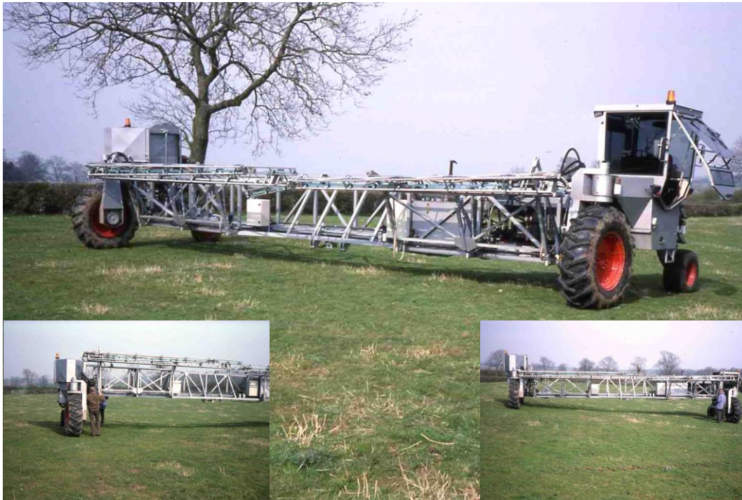
Fig. 7. The second attempt at commercialisation was a machine built by Mel Burrell Fabrications Ltd. The design was based on P1 and although introducing many new features such as centre section height adjustment, it proved too heavy for the power available.
