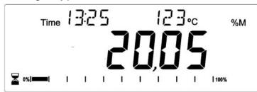
Showing a test in progress for 13:25, with a current temperature of 123°C and 20.05% moisture, the test is still running.
