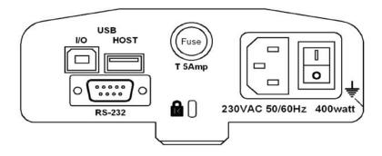
The rear panel has connectors for the data interface, fuse holder, security lock location and power supply input.
