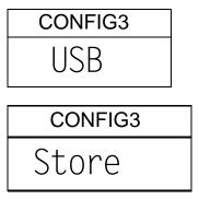
Press [Select] to confirm the action. Or press [Tare] to escape back to the original USB display.
