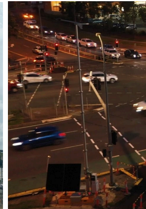
Large Intersection achieved compliant lighting using on 4 x Hammer Head units with 12m Mounting Height and Type 4 Optics
