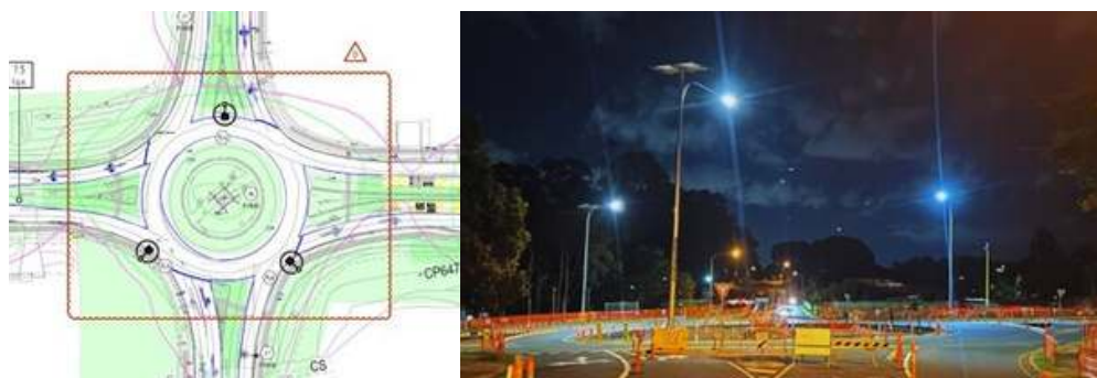
Compliant Lighting Achieved from 3 Outside Locations
