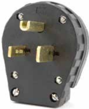
HEAVY DUTY 50 AMP PARALLEL BLADE PLUG PIN-TYPE, 250 VOLT RATED, NEMA 6-50P
