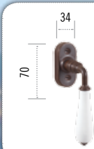
FM 385.DK Mezza martellina D.K. in porcellana con \nabla 7 mm Window handle porcelain dry-keep movement, 4 click positions, spindle \nabla 7 mm
