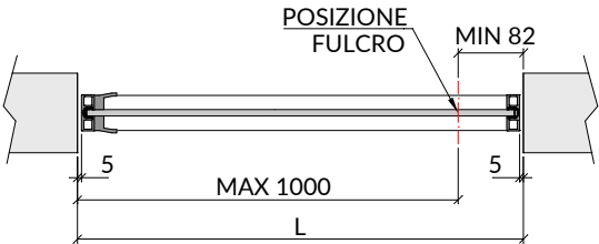
Iris con cerniera a filo anta, muro a vista Iris with flush hinge, exposed wall
