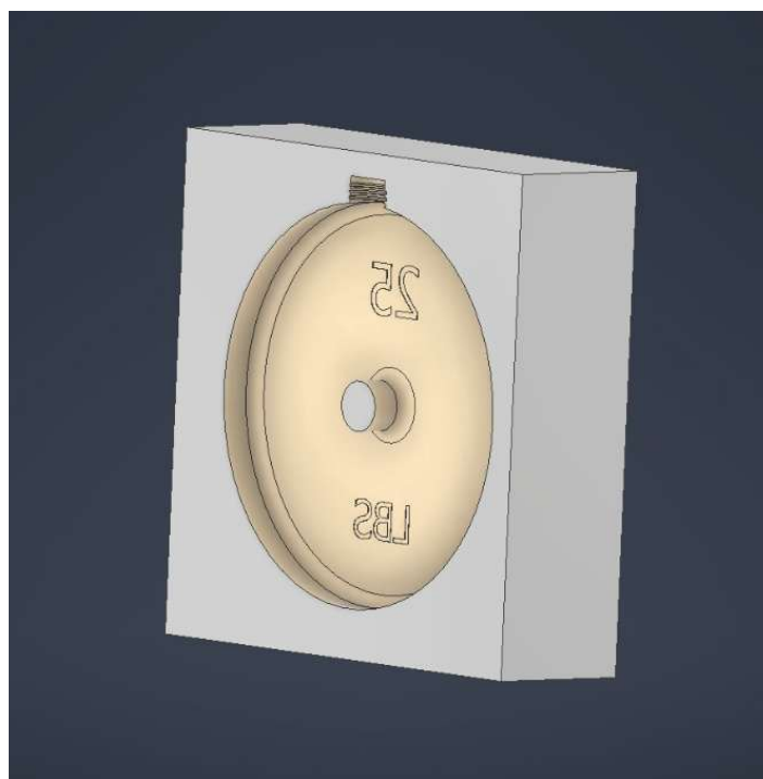
Figure 4: B-half of mold
