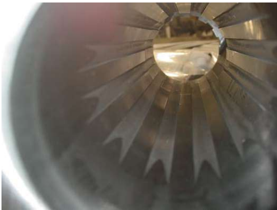
Front view of grooved feed
