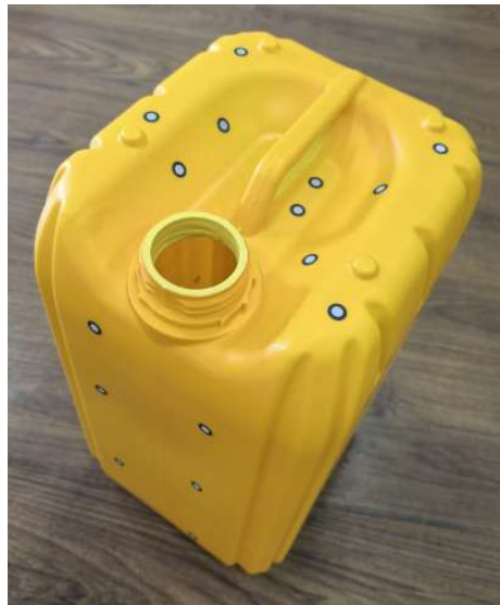
Six-surface marked and SCAN outer surface to create 3D model and 2D drawings
