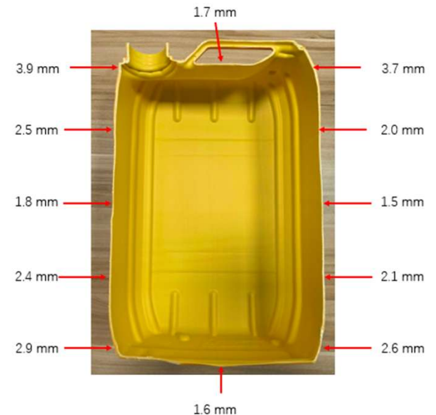
Wall Thickness Measurement
