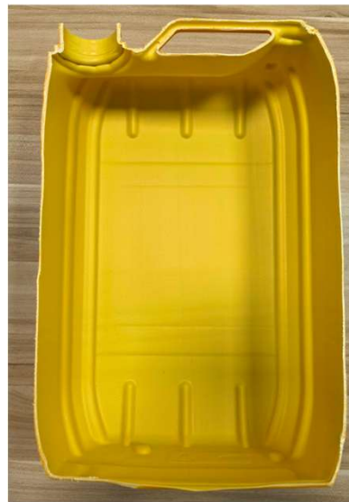
Sectioned and SCAN inner surface to create 3D model and 2D drawings
