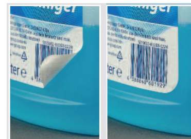
Adhesion of a label with and without the effect of diffusing contents
