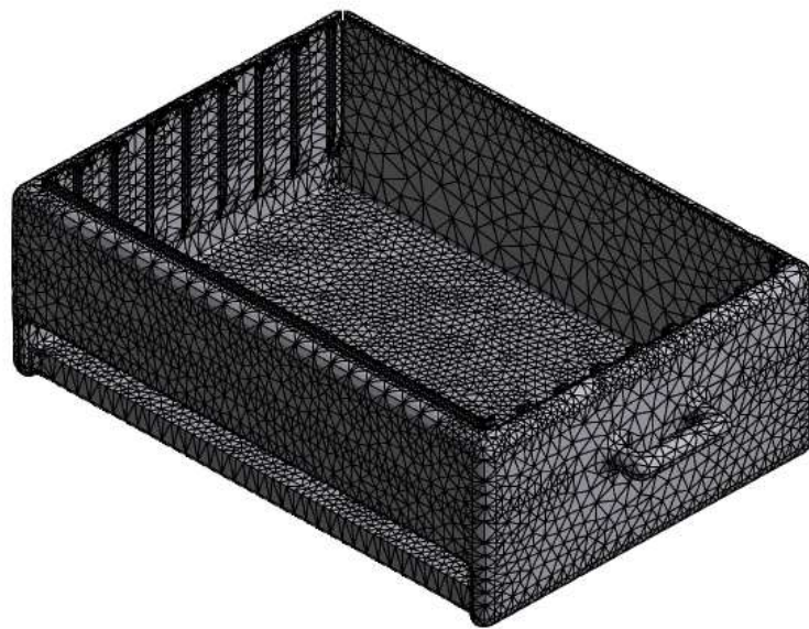
Figure 7: ANSYS Meshing Layout of Bee Box
