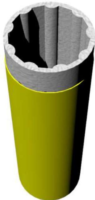
**TUBO FORMA** E' IL MODO PIU' VELOCE PER REALIZZARE DELLE COLONNE SAGOMATE. ESSE SONO REALIZZATE IN DUE PEZZI, IL CARTONE PERMETTE DI RESISTERE SENZA PROBLEMI ALLA PRESSIONE IDROSTATICA DEL CALCESTRUZZO E IL POLISTIROLO FA ASSUMERE LA FORMA DESIDERATA. IN QUESTO MODO OLTRE AD EVITARE L'USO DI CHIODATURE, FASCIAMI, STAFFATURE, PUNTELLI ECC. SI RIESCE AD OTTENERE UN PILASTRO SAGOMATO NELLE FORME CHE OCCORRONO, RISPARMIANDO NOTEVOLI COSTI DI TEMPO E DI MANODOPERA.
