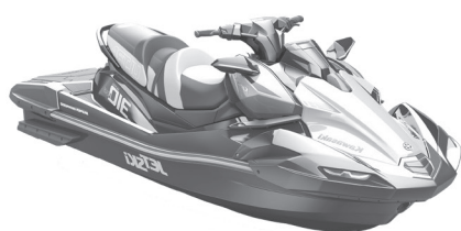
Kawasaki JET SKI 310 ULTRA LX-S featuring a Supercharged 1498 cc engine
