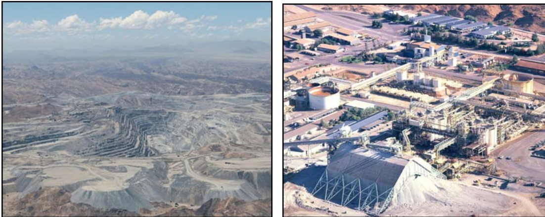
Plate 4.3: Aerial views of Rössing mine and part of the Rössing plant. Much of the total footprint of 24 km 2 is taken up by waste rock dumps (photo SAIEA and Rössing).
