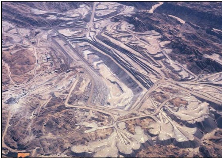
Plate 4.7: The Rössing pit is about 3 x 1.2 km in size, and 345 m deep. This, and the surrounding waste rock dumps, are permanent features that cannot be rehabilitated to the original landscape. The channel of the Khan river is visible top right (photo P.Tarr).
