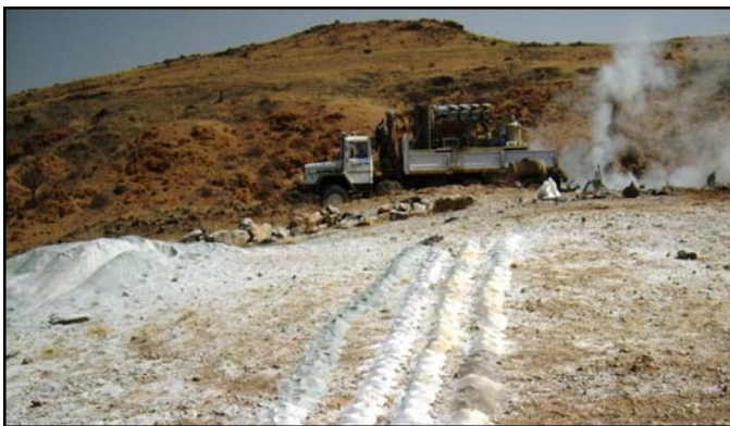
Plate 4.6: Percussion drilling samples during definition of the proposed pit of Valencia mine (photo Geological Survey).
