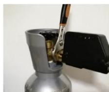
Connect the gas cylinder and valve with a wrench
