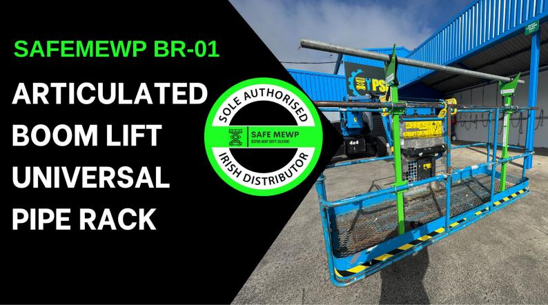
The BR-01 Universal Pipe Rack is designed to fit articulated boom lifts quickly and securely, no tools required. With a 60kg capacity, heavy-duty securing straps, and a low-profile design, it helps operators lift and transport materials safely while reducing manual handling risks. Fits multiple boom manufacturer makes & models
