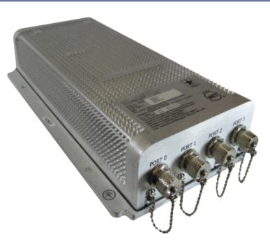
The Multiprotocol Rail Reader (MPRX) is a fully integrated, self-contained 902- to 928-MHz wireless radio frequency identification (RFID) reader that is specifically designed for rail applications.
