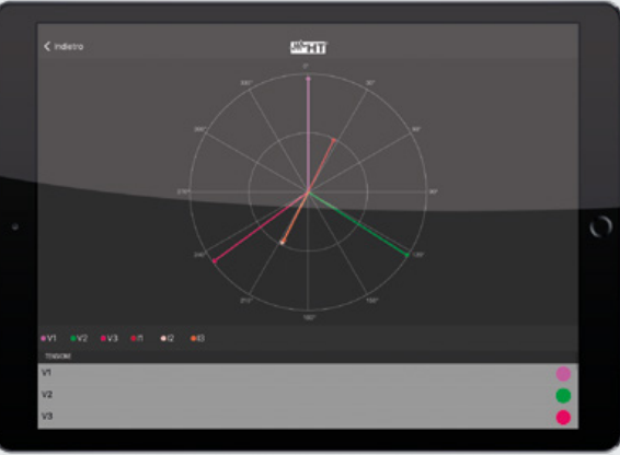
Voltage and current vector diagram.
