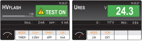
Dielectric strength test.
