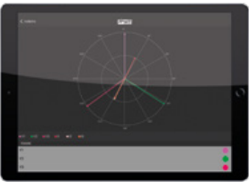
Example of display Real-time phasors
