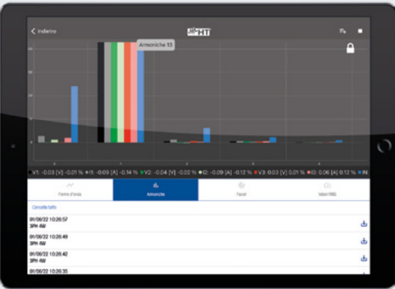
Current and voltage harmonics.
