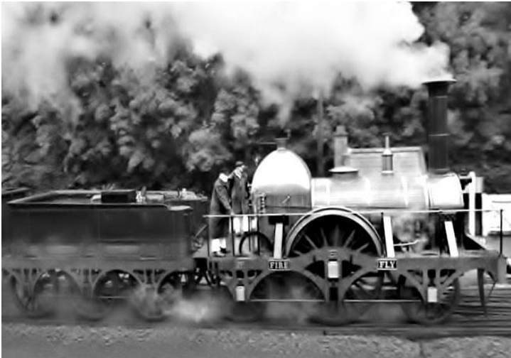
'Fire Fly': A broad gauge replica loco, completed at Didcot Railway Centre
