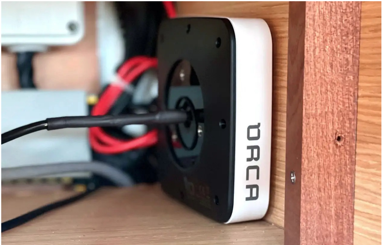
Orca Core installed with the bonding pad. The drill-through mount is removed.
