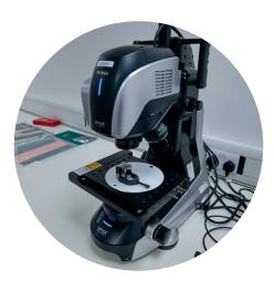
An advanced 4K, high-accuracy microscope that allows for highmagnification imaging and measuring of samples with magnification over 2,500x. Z-stacking allows for full image focus of uneven samples and can generate 3D renders based on topographical height. Additionally, it is able to do 2D and 3D measurements of samples including surface roughness profiling. Optical shadow effect mode allows for SEM-like surface detailing without the hassle.
