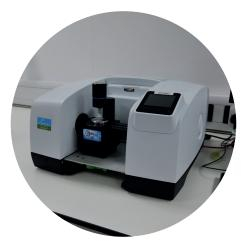
The FTIR spectrometer directs infra-red light towards the sample, where the chemical bonds in the sample absorb the light at varying frequencies. Measuring the light across the spectrum enables the sample to be identified.
