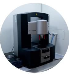
The rheometer is used to measure the flow properties of a sample material to understand how it may move through a production process. Using both rotational and oscillatory testing, various material parameters can be determined, including viscosity at varying shear rates, viscoelastic behaviour, relaxation times, shear stress and strain, and more.
