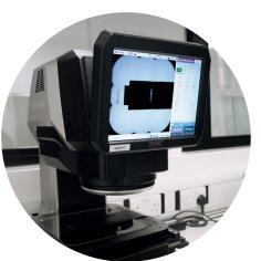
The shadowgraph uses light beneath the stage and a high-density camera to measure mechanical parts. Telecentric lenses use mean high accuracy measurements with no drift. In addition to the standard shadowgraph, it has:
