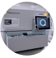
X-Ray diffraction (XRD) is a nondestructive analytical technique used to obtain information about the chemical composition and crystal parameters of a sample, including structure, orientation, and size.
