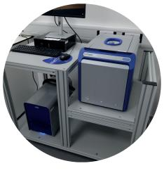
The Nuclear Magnetic Resonance (NMR) spectrometer is acompact, high performance system for fast analysis of liquids and gels. It does not require cryogens and features a high-homogeneity, permanent magnet for exceptional temperature stability.
