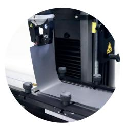
Tensile testing evaluates the mechanical strength of a material through tension or compression of the material until breaking point. It can also check the force required to separate two joined components.
