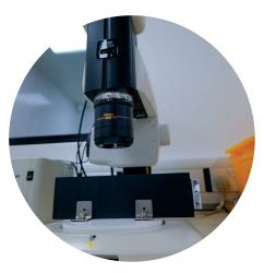
The optical microscope uses visible light and a series of lenses to magnify a sample to enable the viewing of surface features. The microscope is fitted with a camera to enable images of samples to be taken and analysed. In the current configuration the microscope can magnify to 150x – other objectives can be purchased to achieve higher magnifications.
