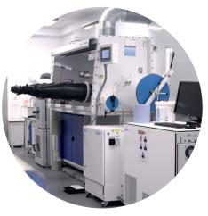
An argon-filled glovebox for smallscale building of cells, particularly, half-cell coin cells.
