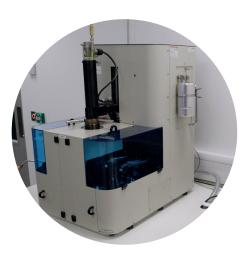
Mercury porosimetry is used for measuring pore size distribution within a solid material.
