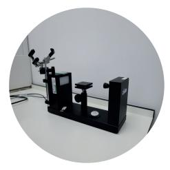
The Ossila contact angle goniometer measures contact angle and surface tension of liquid droplets. The droplet can be put onto any surface to measure the interaction of the liquid with the surface of interest.
