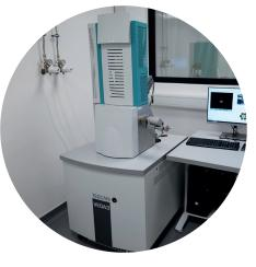
The scanning electron microscope (SEM) uses electrons to view a sample in opposition to light.
