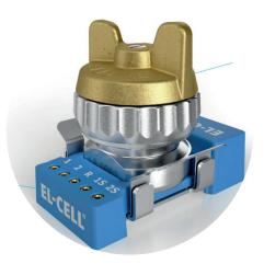
We have six cells that can be connected to our potentiostat via the PAT-Clamp-1 docking station for electrochemical analysis (cycling testing, EIS compatible). It can also be used inside the environmental chamber and operate in temperatures from -20 to 80°C. The maximum electrode diameter is 18mm and the maximum separator diameter is 21.6mm.
