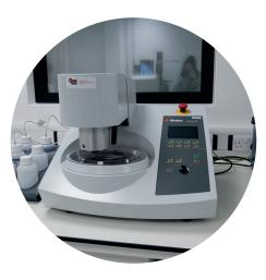
Mechanical polishing is used for the grinding and polishing of the crosssectional surface of resin mounted samples, resulting in a smooth and even surface so that surface features can be clearly seen under the microscope or SEM.
