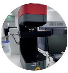
Hardness testing measures a material's resistance to permanent deformation at its surface, using an indenter that presses into the sample for a few seconds with a specific load behind it.
