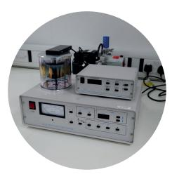
Samples for the scanning electron microscope (SEM) must be conductive. For samples with low or no conductivity, the sputter coater can be used to cover the samples in a thin conductive layer (~10nm). This is needed for all samples that have been mounted in non-conductive resin.
