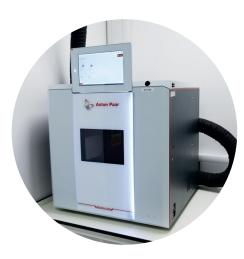
The microwave digester is used to heat solid samples, typically in an acid medium, in a sealed vessel using microwave radiation which quickly raises the temperature and pressure. This rapid heating breaks down the sample much faster than the traditional method of using a hot plate.
