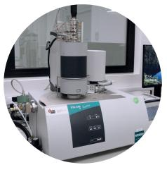
Simultaneous Thermal Analysis (STA) enables simultaneous running of thermogravimentric analysis (TGA) and differential scanning calorimetry (DSC) on samples.
