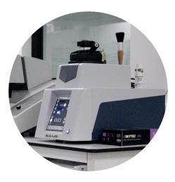
Cold mounting is done using epoxy resin and hot mounting uses the Buehler Simplimet 4000. Samples are mounted to see the cross section of materials for further analysis.
