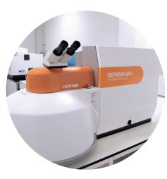
Raman spectroscopy is a chemical analysis technique that involves illuminating a sample with laser light and measuring the scattered light from the sample's surface. The scattered signal provides valuable information about the composition and structure of the material.
