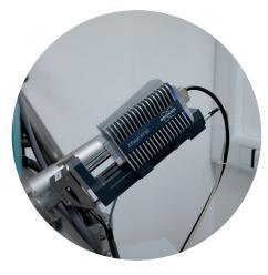
Energy Dispersive X-Ray (EDX) spectroscopy allows the user to analyse the elemental composition of a sample by detecting characteristic x-rays emitted by the elements in the sample. When working alongside SEM, EDX can be used to create elemental maps of samples.
