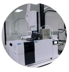
Gas Chromatography - Mass Spectrometry (GCMS) separates volatile components in a mixture to enable them to be identified.
