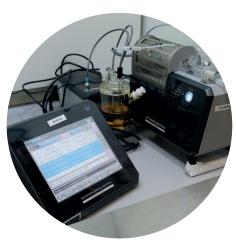
The Karl Fischer titrator determines the moisture content of a sample based on the reaction:  $I_2 + 2H_2O + SO_2 \rightarrow 2HI + H_2SO_4$
