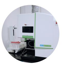
Inductively Coupled Plasma Optical Emission Spectroscopy (ICP-OES) is used to determine how much of an element is present in a sample.
