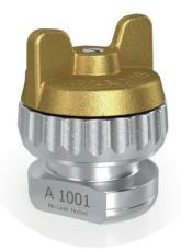
PAT-cell is a test cell for 2- and 3-electrode high-throughput battery testing for extended time periods (>1000 hours). It is designed for easy handling and fast assembly and can be used inside the glovebox. The cell is compatible with both aprotic and aqueous electrolytes.
