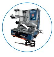
A semi-automatic 'Z' fashion stacking machine designed to alternately stack anode and cathode electrode sheets with a separator film in between.
