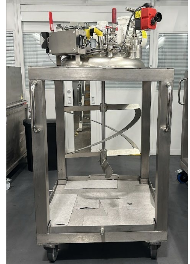
Cups (left) vs helical (right) agitator design
