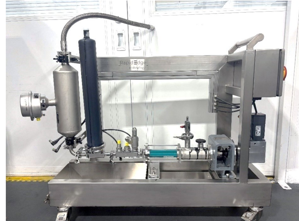
Streamlined slurry delivery system at UKBIC with 17 connections . With inline gauges, reduced number of clamps and a purge valve immediately prior to the pump. Mechanical seal pump
