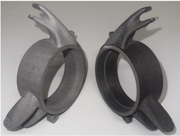
Figure 18: Mirrored LPBF builds and the calliper-mount deformation observed on Build 2: Build 1 (left, bead-blasted) and mirrored Build 2 (right, as-built).
