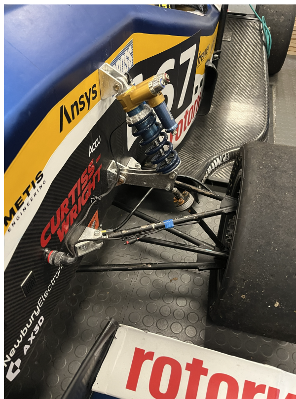
Figure 1: Double wishbone set-up on TBrE25
