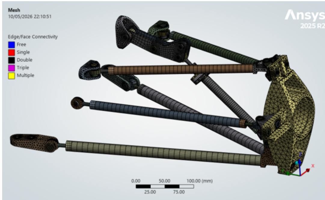
Figure 12: Final mesh of full suspension system
