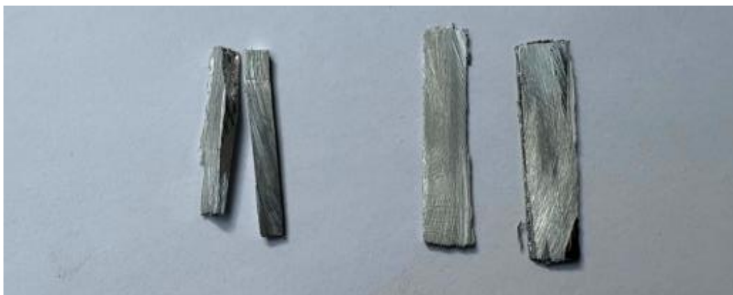
Figure 18: Aluminium samples; 7075 on the left, 5083 on the right.
