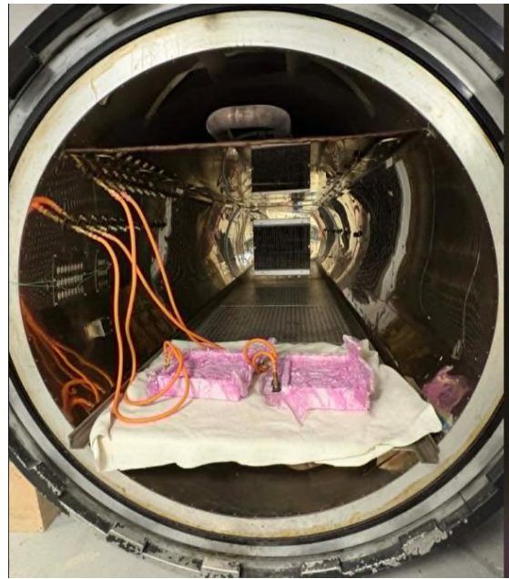
4. Once fully laminated the moulds were bagged and cured in an autoclave at 60deg for 12h at 90psi pressure.
