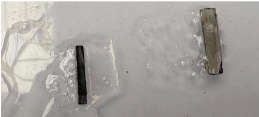
Figure 19: Reaction of sample; 7075 on the left, 5083 on the right.
