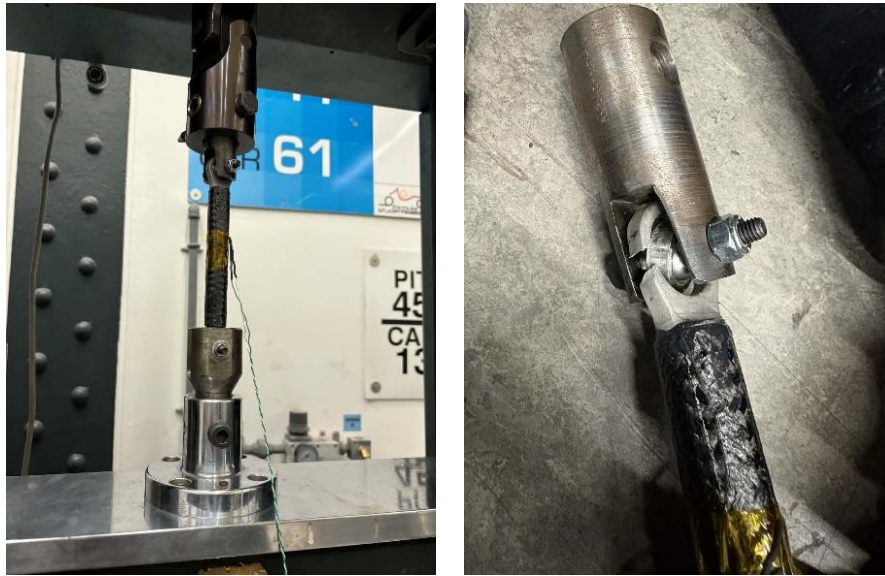
Figure 16a: Tensile test setup and material failure.
