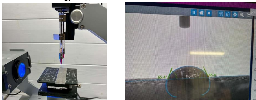
Figure 13a: Contact angle measurements using DSA - Contact Angle and SFE analyser
