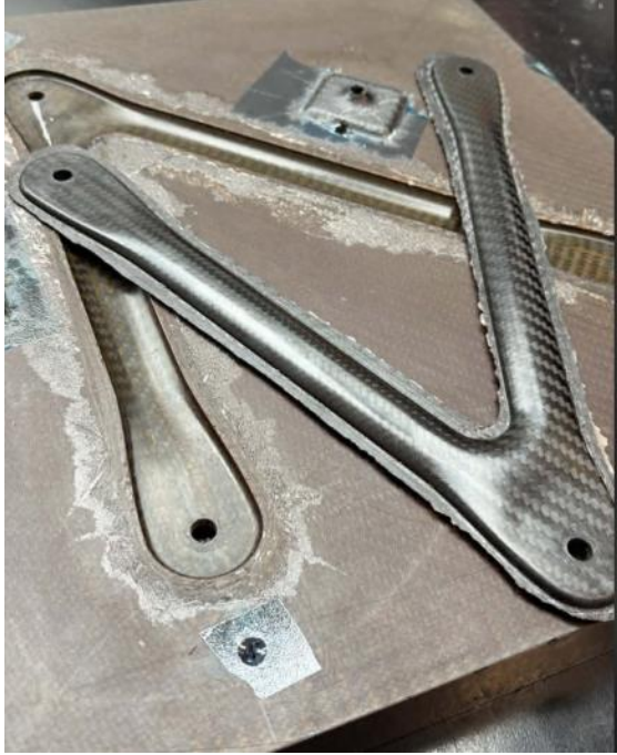
7.Cured wishbone half. The machining of the wishbone is then carried out according to the processes outlines in Appendix F.
