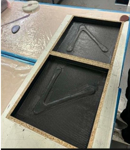
3. Carbon moulds prior to the addition of laminating bushes.
