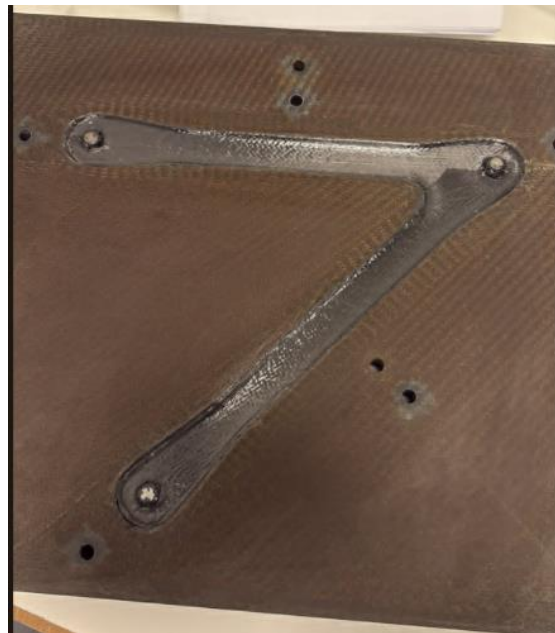
6. The mould was sealed and release. Lamination as per laminate book in appendix E began.
