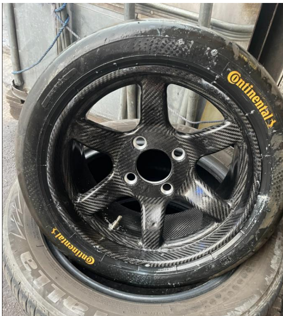
Figure 95 - Tyre fit and inflated onto rim - post leak test - dunk tank seen in background
