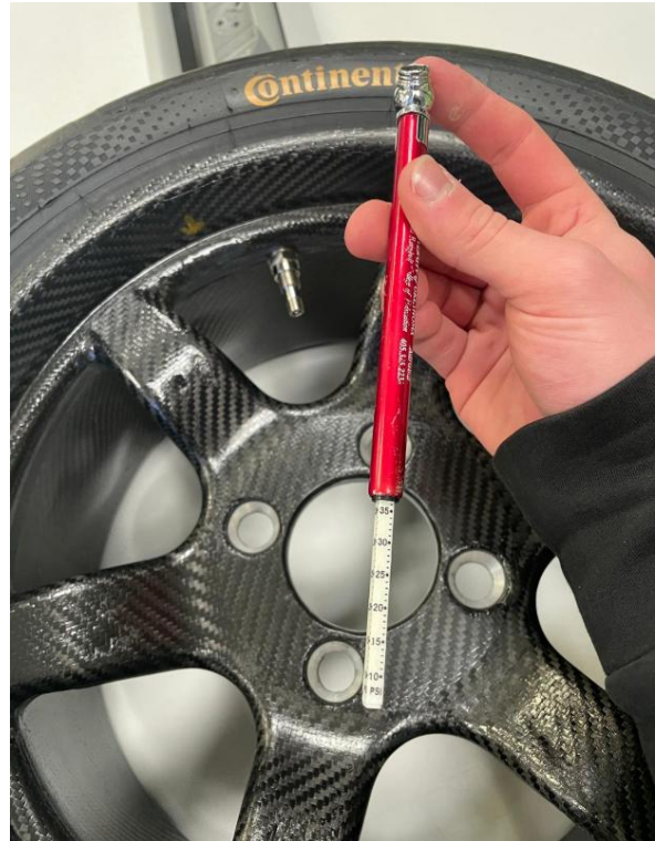
Figure 98 - Final day (7) of pressure test - reading 36.5psi
