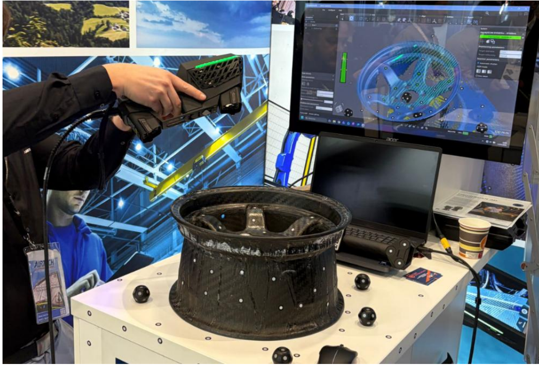
Figure 88 - 3D blue light scanning of Variant 2 CFRP wheel rim for dimensional inspection
