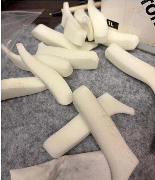
Figure 66 - Machined foam core for variant 2
