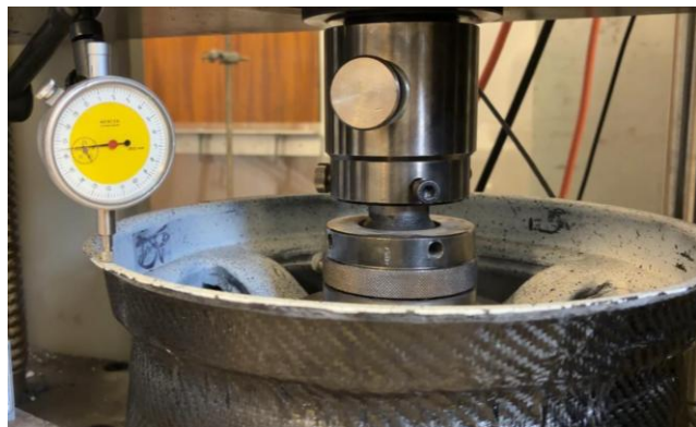
Figure 109 - Variant 1 (no core) under axial loading
