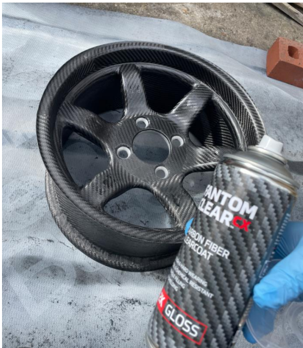
Figure 81 - application of the Phantom Clear UV resistant coating
