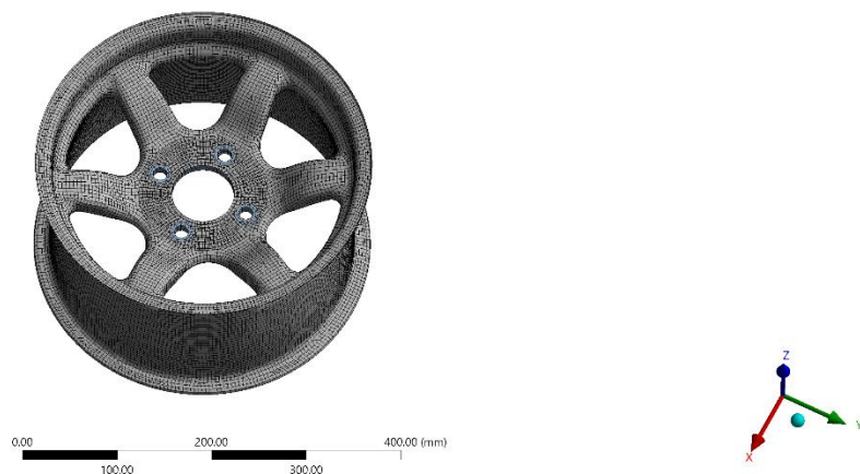
Figure 39 - Initial total assembly mesh of 30k elements
