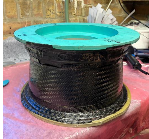
Figure 76 - First layer after combining the two mould halves
