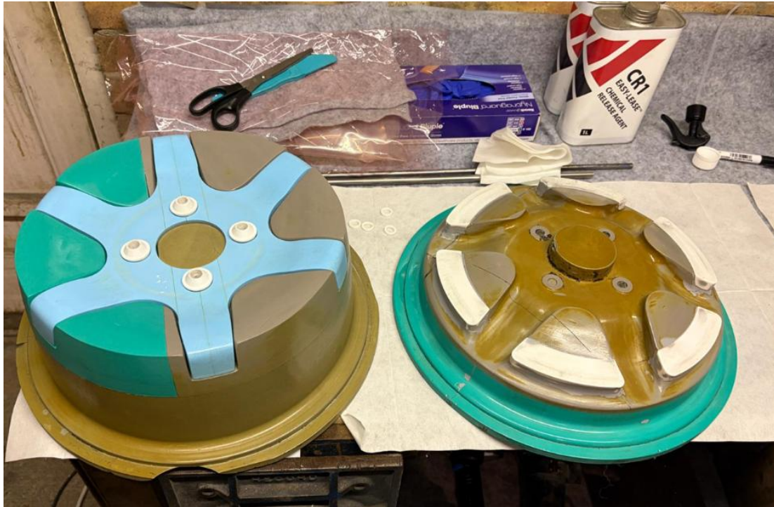
Figure 72 - Variant 2 moulds, blue interchangeable mould swapped and inserted into upper mould (left hand side)
