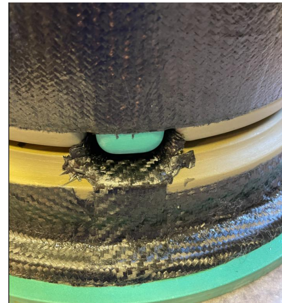
Figure 71 - Variant 1 - mould closure
