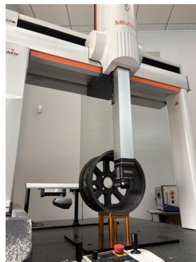
Figure 15 - Dimensional checks using a CMM
