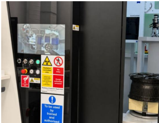
Figure 102 - Wheel going into the CT scanner
