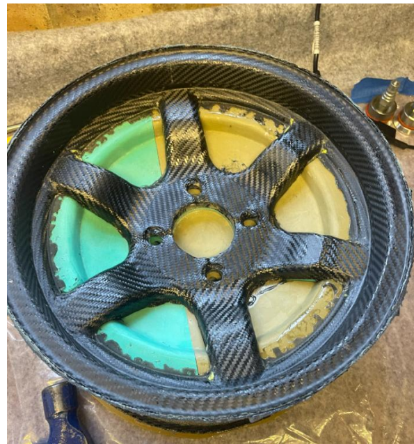
Figure 78 - Lower mould removed, post cure
