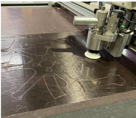
Figure 64 - Cutting carbon plies using a 3-axis plotting cutter
