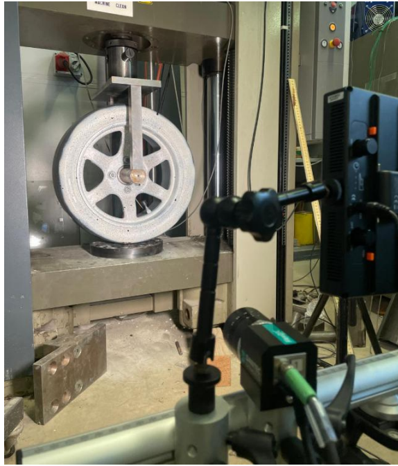
Figure 12 - Physical test setup, testing radial loads
