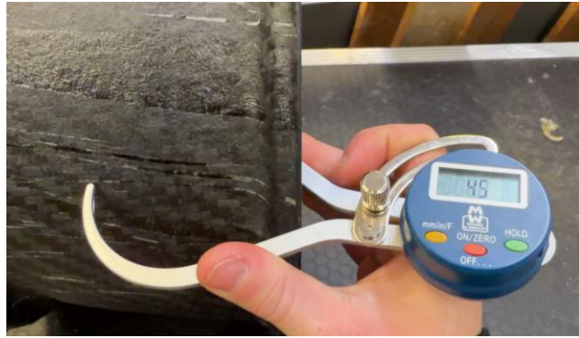
Figure 85 - Measuring barell thickness
