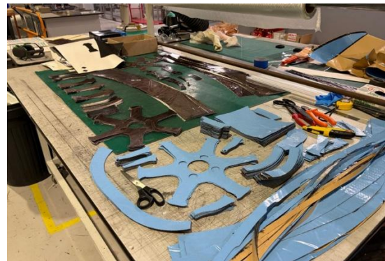
Figure 65 - All 319 plies cut and organised (both ud & woven carbon fibre)
