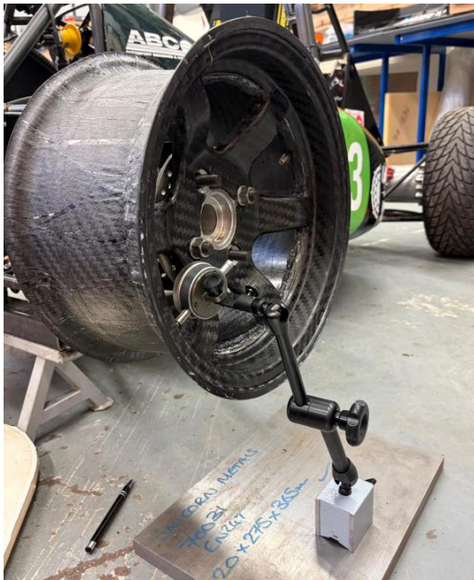
Figure 86 - CFRP wheel fitted to the front suspension for run-out measurement
