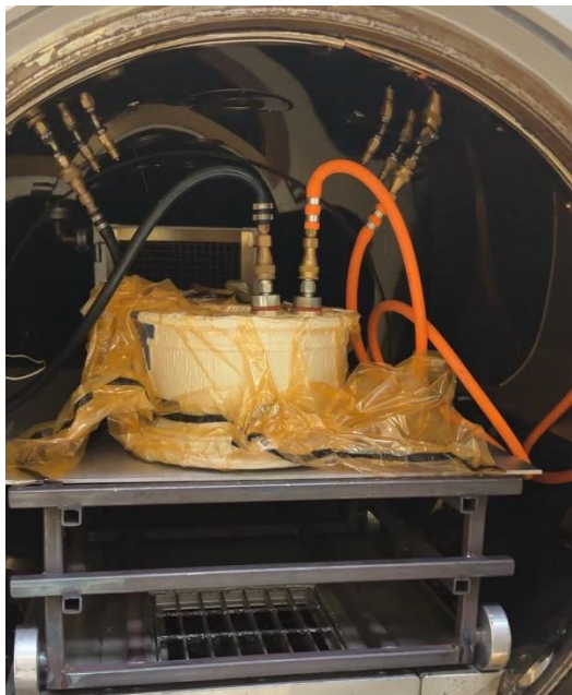
Figure 77 - Autoclave curing (3 hour dwell at 135C, 1 degree C ramp up and down)
