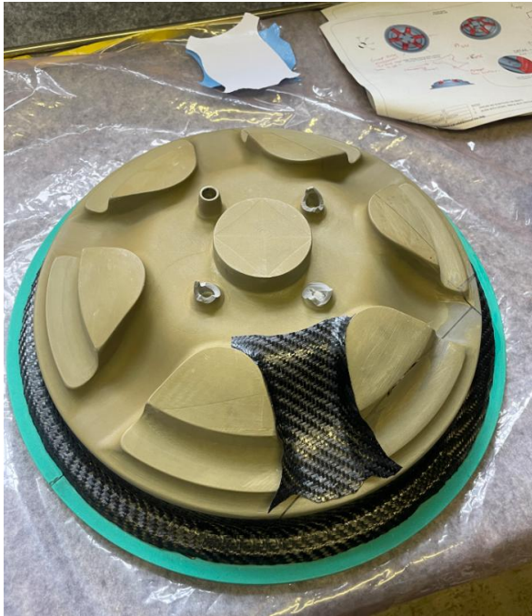
Figure 68 - Variant 1 - first layer of woven carbon
