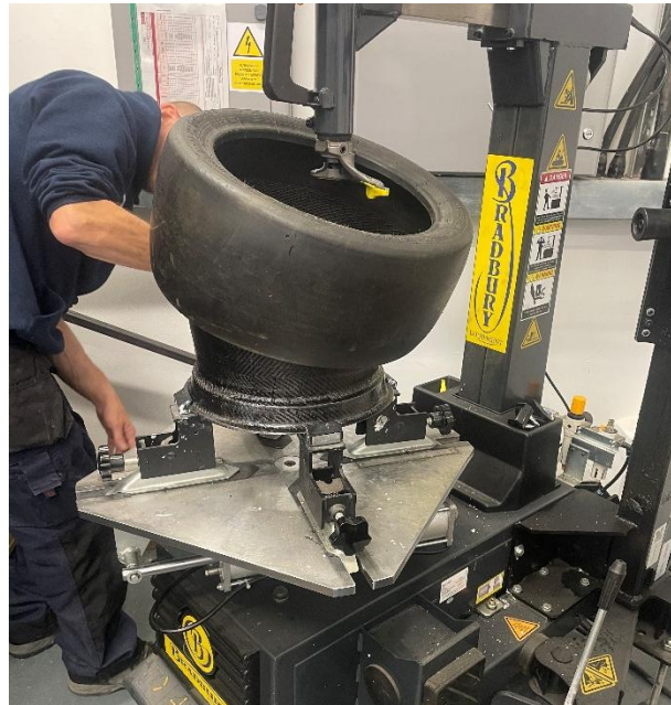
Figure 94 - Tyre fitment (205/470R13 34M slick) using a tyre changing machine
