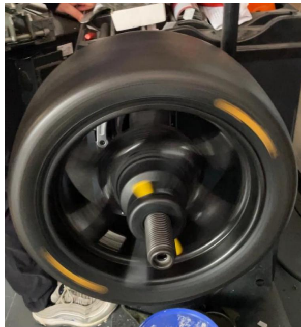
Figure 96 - Wheel and tyre assembly on wheel balancer
