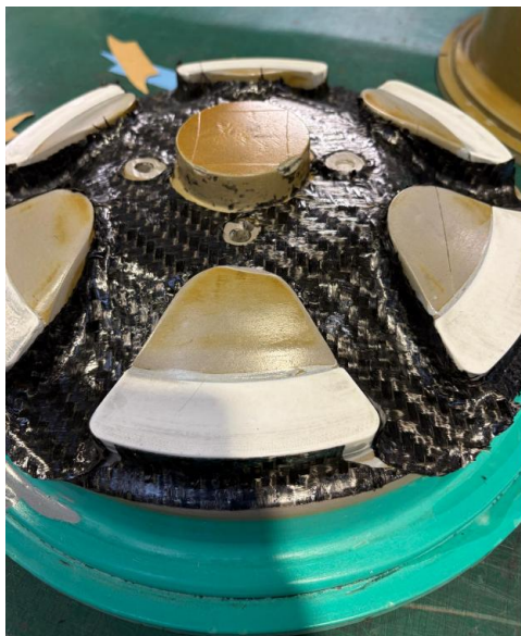
Figure 73 - Variant 2 (foam core) first layer placed into mould - Woven
