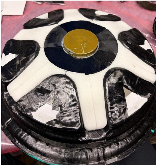
Figure 75 – Variant 2 (foam core) placing the rest of the foam core – typically left empty with variant 1 (no foam core)
