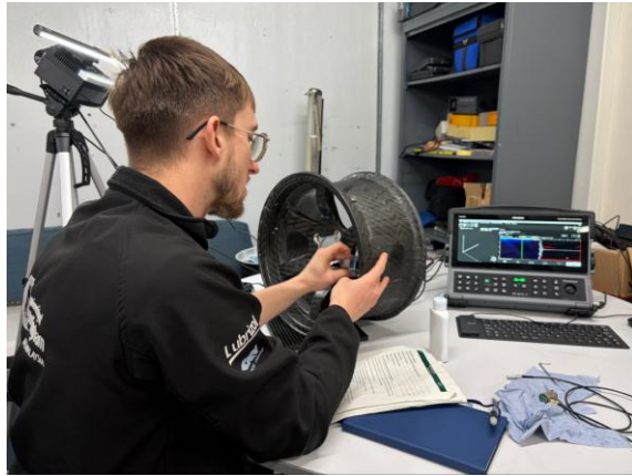
Figure 99 – Ultrasonic test setup with probe detector
