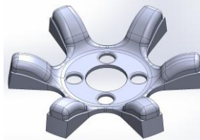
Figure 52 - Interchangeable centre for C-channel (no foam) variant
