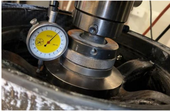
Figure 110 - Close up shot of test rig, dial indicator measuring spoke deflection
