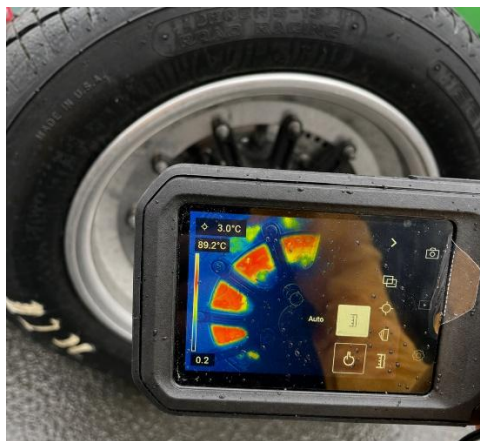
Figure 113 - 21/09/2025 thermal imaging (via FLIR) post endurance test running
