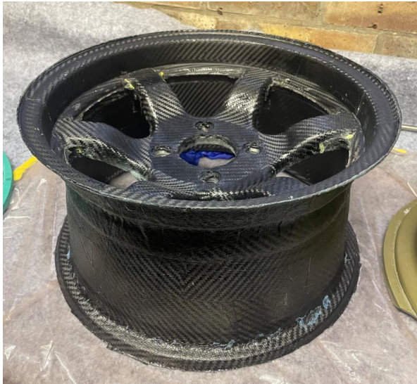
Figure 79 - Demoulded wheel, pre trimming
