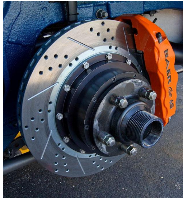
Figure 9 - Centre Locking assembly
