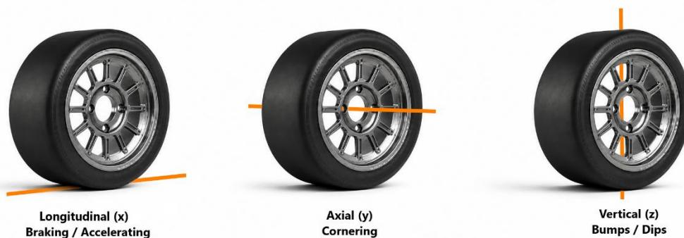
Figure 28 - Axis and load directions
