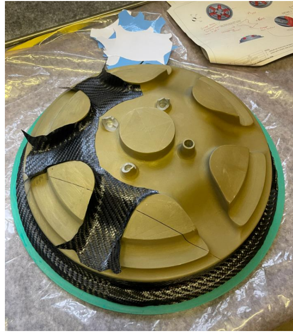
Figure 69 - Variant 1 - laminating of remaining spokes
