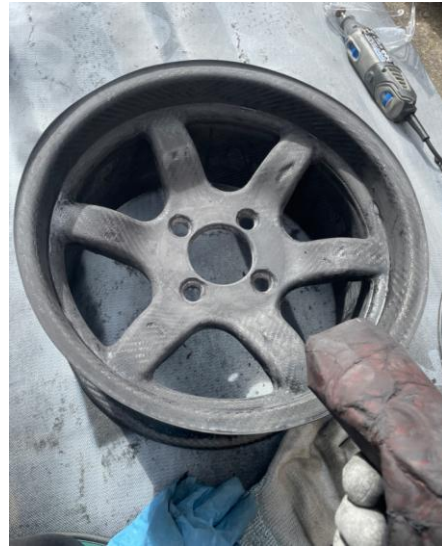
Figure 80 - Post cure trimming, sanding & polishing
