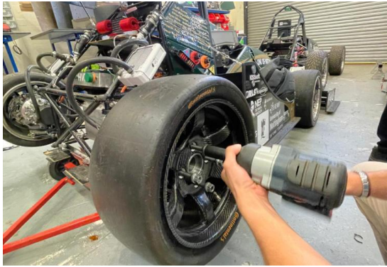
Figure 84 - Fitting wheel and tyre assembly onto the FS25 racing car
