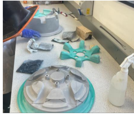
Figure 63 - Sanding, sealing and releasing the moulds post machining
