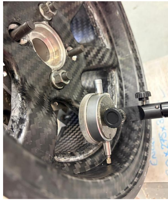
Figure 87 - Close up showing dial indicator sweeping inner bead surface (external surface is too rough for useful readings)
