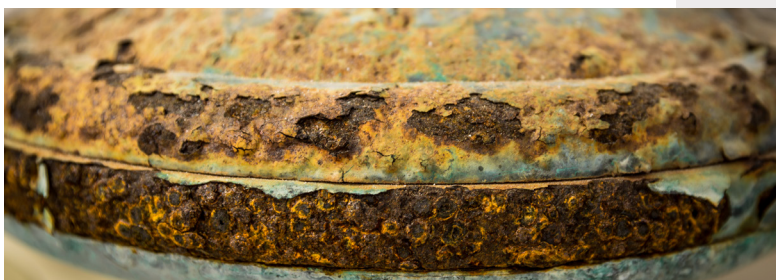
CORROSION OF AN OUTDOOR FIXTURE
