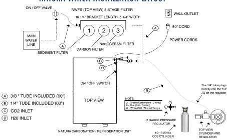
NOTE: IT IS RECOMMENDED TO HAVE THE FOLLOWING CLEARANCE AROUND AND ABOVE THIS UNIT: 6" SIDE, 2" BACK, 6" TOP
