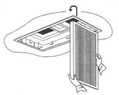
15. To ensure air flow through the filter is in the correct direction. Install the filter/s with the recess part of the filter facing down.
