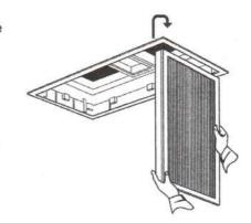
13. To install grille core after cleaning, lift up into return air box pull foreword and allow to drop gently.
