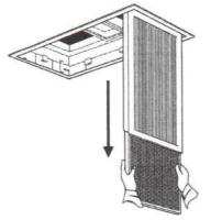
7. If a fresh air filter is fitted turn clips through 90° and remove filter.
