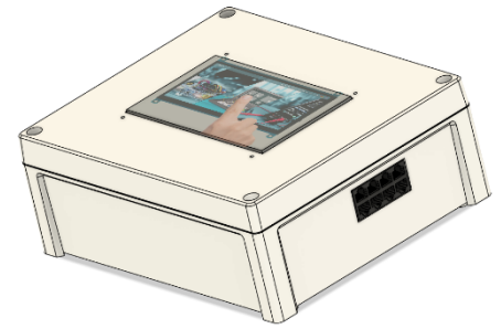
DAQ Enclose with touch display and IO-connection Size (mm) 289x1239x107
