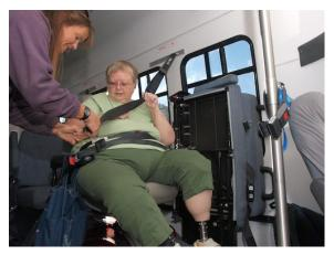
In addition to a securement system for the mobility device (wheelchair), vehicle standards in 49 CFR Part 38 require a seat belt and shoulder harness for the user of the mobility device. Such seat belts and shoulder harnesses must never be used without also ensuring that the wheelchair itself is secured Section 38.23. Transit agency personnel must assist with securing the seat belt and shoulder harness upon request as part of the overarching requirement to make use of the accessibility features.
