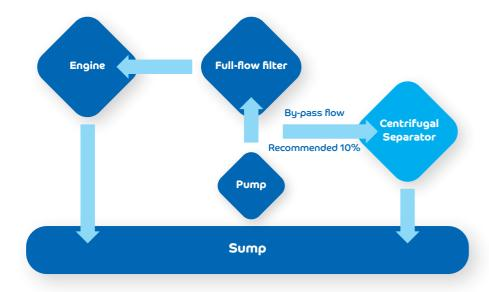
Smaller sub micron particles pass through the filter media continuously.
