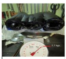
2.7kgs sludge in 200 hours. Equates to 13.5g/hr.
