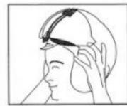
Helmet wearing is given by the low position of the inner visor.
