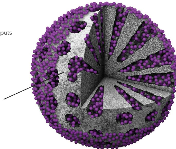
Ions of the **crop protection** solution are attracted to nanoparticles, filling the empty space and also forming an outer layer of ions around the nanoparticle. Loaded particles are now ready for effective delivery.
