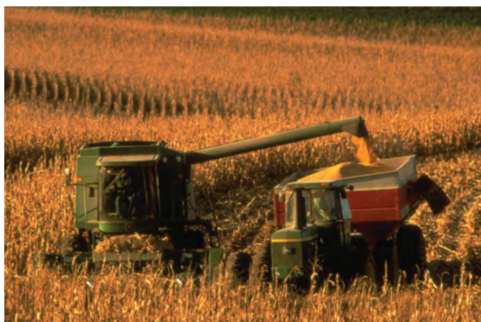
Figure 12. Two-wheeled grain carts with unload augers were an important innovation that increased the speed and efficiency of harvesting higher-yielding corn.
