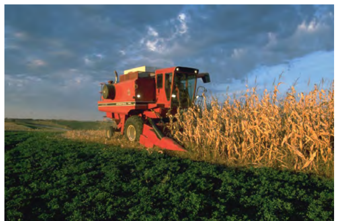
Figure 11. International Harvester axial-flow rotary combine introduced in the late 1970s.
