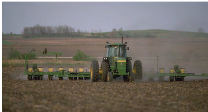
Figure 9. During the single cross hybrid era, corn planters increased considerably in size, efficiency, and accuracy.
