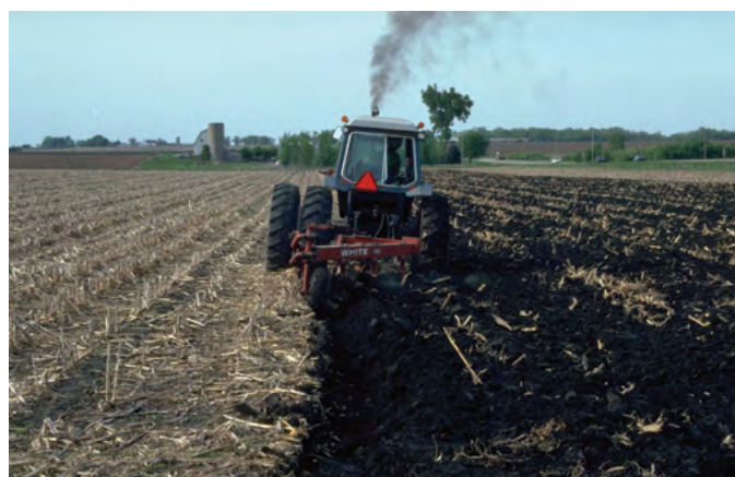
Figure 8. The 1970s and 1980s saw a shift away from intensive tillage using implements such as the moldboard plow shown here and greater adoption of reduced tillage and no-till.
